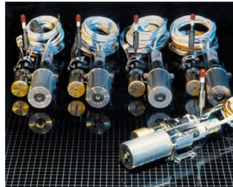
First shipset (plus a spare) Electrothermal Hydrazine Thrusters
